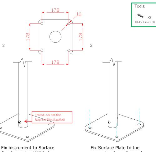
fix plate using M10 bolt and Barrel Nut and use thread locking solution to prevent fixings working loose.
