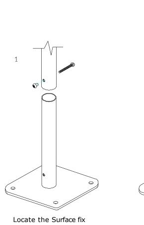
Plate into the leg of the instrument.
